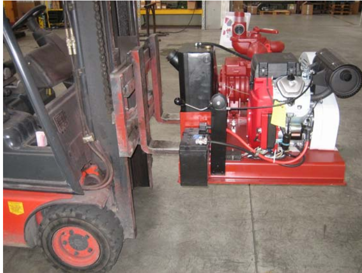
Picture 1: Raising of the engine driven system
